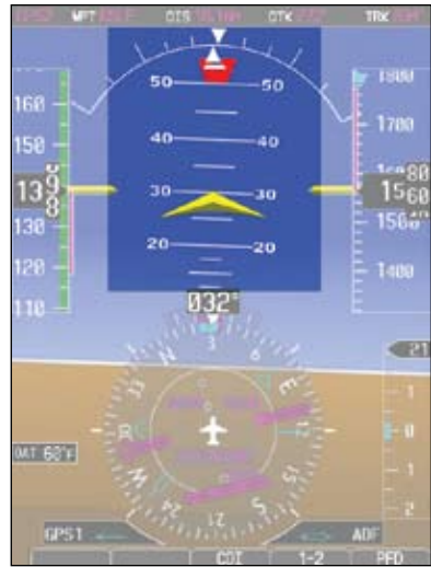
Figure 2-16 Extreme Pitch Indication Nose Up
